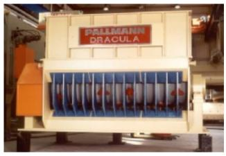
For crushing of soft to medium hard materials, PALLMANN offers a wide variety of single, double and multiple shaft crushers, safety crushers, precrushers, cam breakers, finger breakers, lump breakers, bale openers, drum shredders and roller mills with serrated and smooth rolls. Depending on the application on hand, these machines are supplied with a split housing, external bearings and packing glants.
