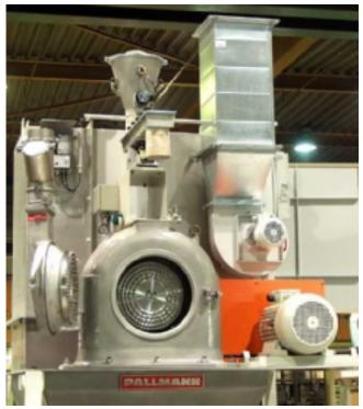
Universal Mills, type PX are used for disagglomeration, preparing, coarse, medium fine up to 5 micron. All soft to medium hard materials (hardness 3 according to Mohs) for dry, moist or wet grinding, even of fatty, adhesive materials.
