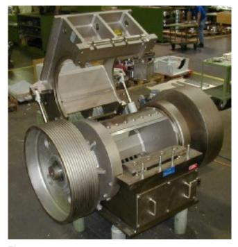
PALLMANN supplies complete lines of granulators, chippers and knife mills for the size reduction of materials which can be cut. Depending on the type of material and the requirements, different infeed systems are to be used: belt conveyor, feed rollers, load controlled feeding with vibratory feeder. The machines are equipped with open or closed rotors with straight cut, slanted cut and scissors cut.
