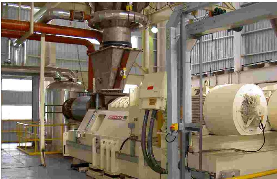
Inside the chip bin the wood chips are preheated by steam alternatively temperature or mass flow controlled. The 20" plug screw feeds reliably chips to the digester and balances the moisture. Pre-heating time in the digester is automatically controlled by the radiometric level control and as a function of the throughput.
