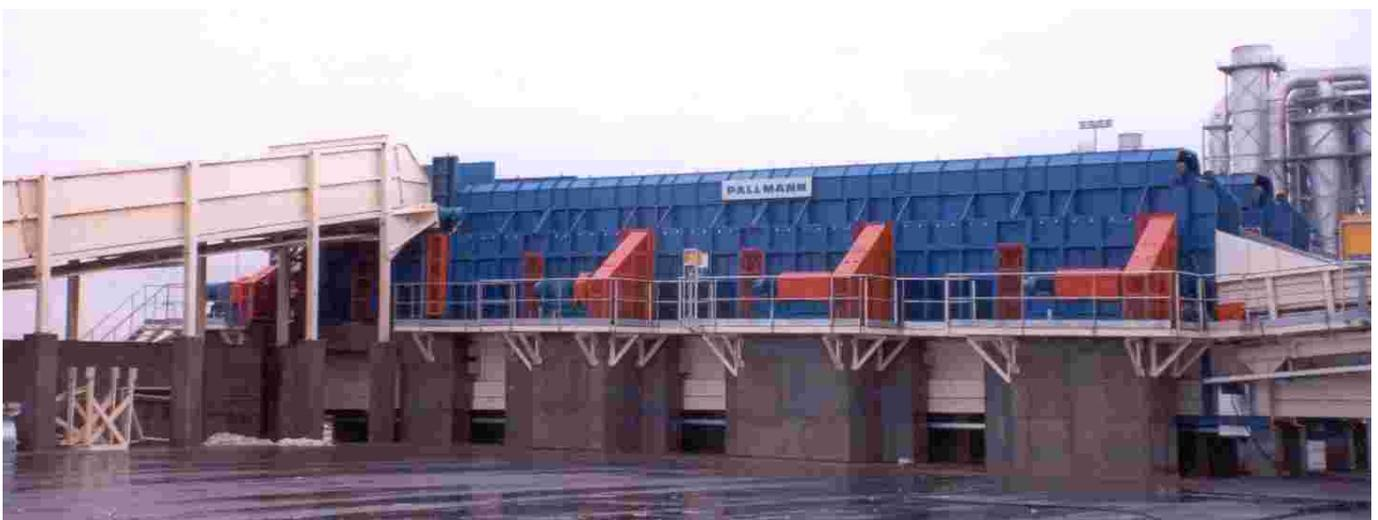
The PALLMANN Rotor Debarker PRD is designed for debarking logs for the MDF / HDF and OSB-industry as well as for all other processes that require thoroughly debarked logs.
