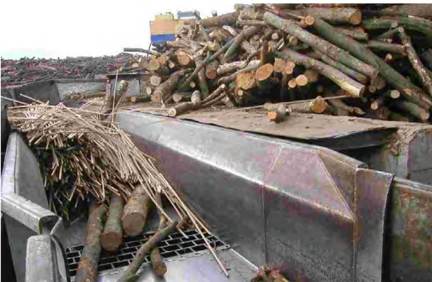
PALLMANN Drum Chippers type PHT produce high quality chips from long and short logs, slabs, edgings, thinnings, veneer waste or board trims.
