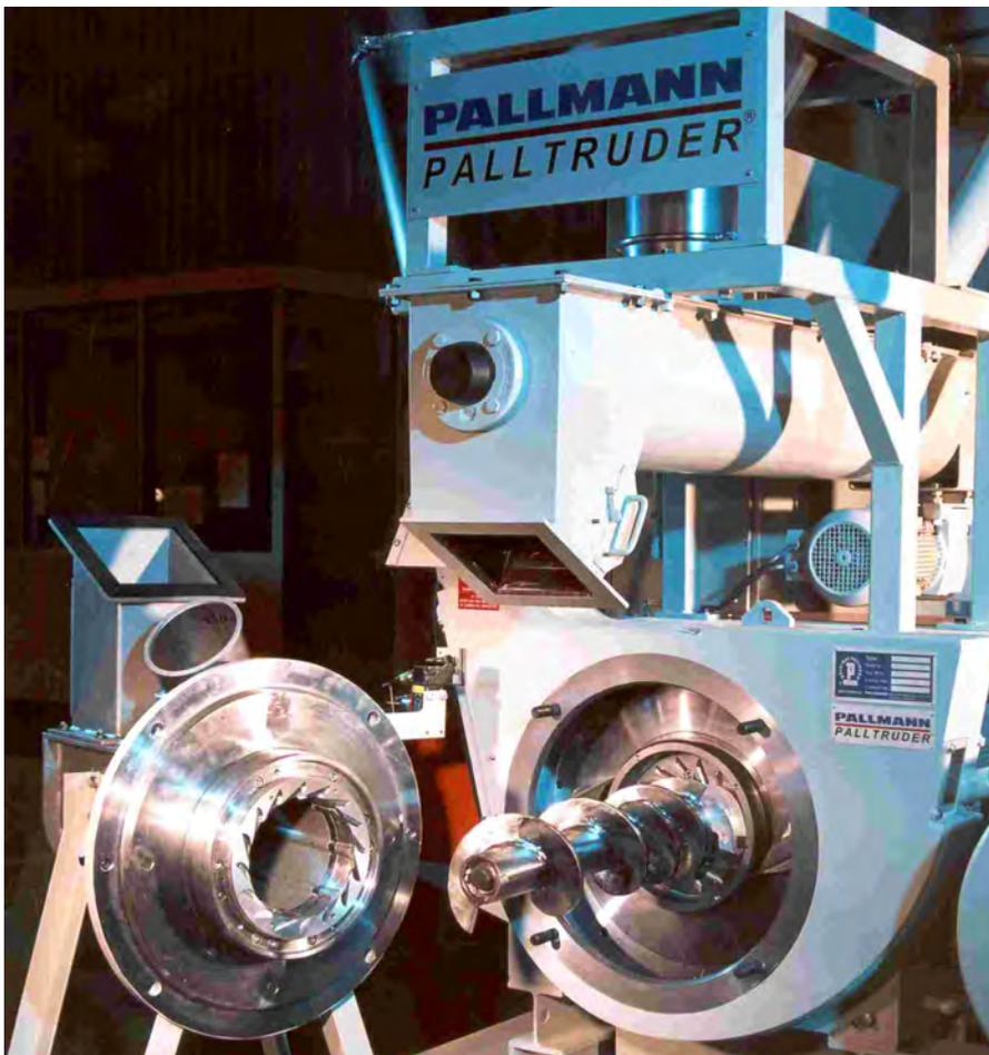
into high quality end products. Four main processing steps characterize Palltrusion™ technology: Metering of the components - natural raw material, plastic and additive, palltrusion, cooling and screening.
