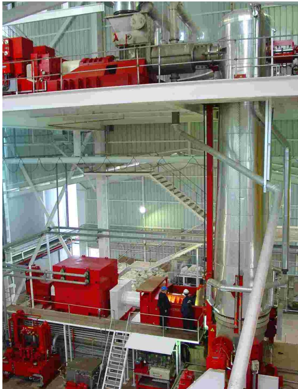
The debarking of round wood is made by the rotor- or drum debarker and the preparation of chips with the approved drum chippers or alternative disc chippers.
