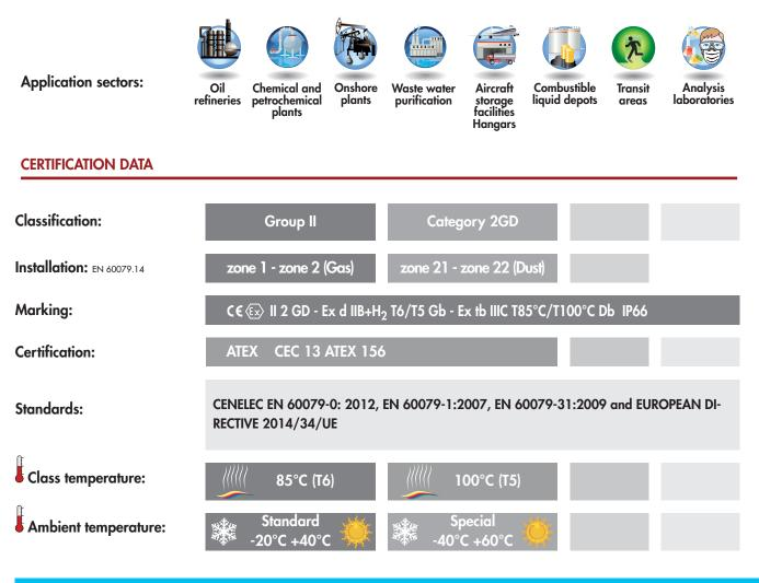
This equipment can be used in an environment containing explosive atmosphere and with the presence of hydrogen.
